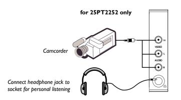
For more convenient direct playback connections, the Side Audio/Video Input sockets allow for quick and easy connections, particularly Camcorder tape recordings.
